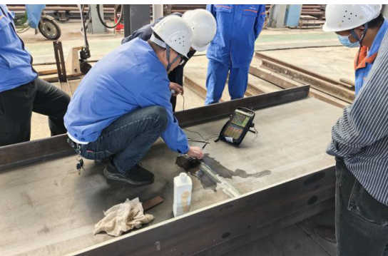
Ultrasonic testing of roof beam welds
